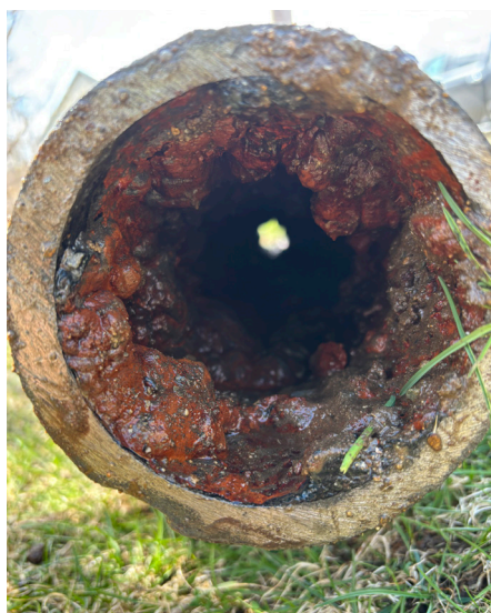
Tuberculation build-up in a water pipe.
