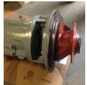
Impeller coated with ceramic protectant.
