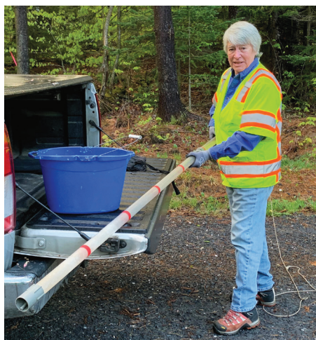
Elizabeth Walker preparing to take samples from a pump station using a sludge judge.
