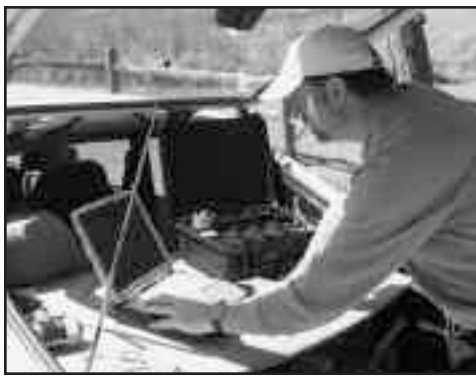
VRWA Circuit Rider, Brent Desranleau uses a leak correlator to help a water system in Manchester, VT. This piece of equipment was funded by a grant from Efficiency Vermont.
